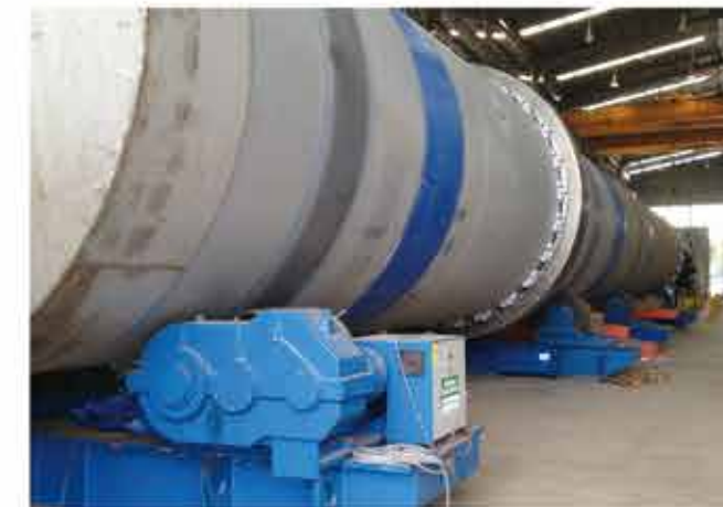
600吨可调式滚轮架（钢胶结合轮） 600t conventional rotator (Rubber+steel ring wheel)
