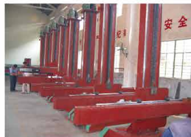
批量生产的精密型焊接操作机（采用滚珠直线导轨） Precise welding manipulator in batch production (uses ball bearing linear guide rail)
