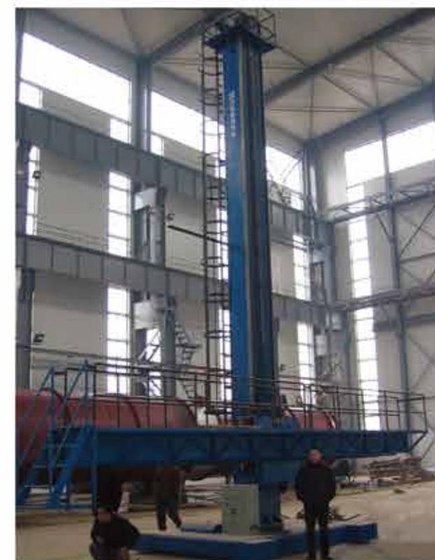
8m×7m超重型焊接操作机（带载人操作平台） 8m×7m super-heavy type welding manipulator(with manned platform)
