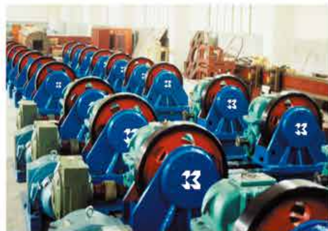
批量生产的窄轮滚轮架（锅炉厂专用） Turning-roll of narrow roll in batch production(specialized for boiler factory)
