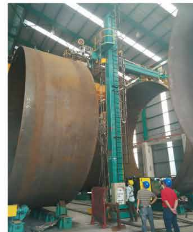
10mx6m超重型焊架 (配伊萨ICE四丝埋弧焊) 10mx6m welding manipulator (Equipped with ESAB ICE SAW)
