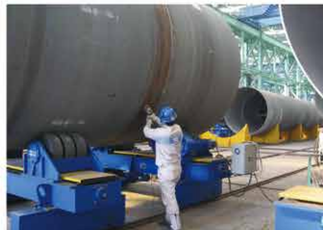
200t可调式焊接滚轮架（聚氨酯轮、电动行走） 200t conventional rotator (PU type, motorized bogie)
