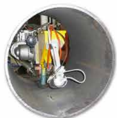
小机头 (适用筒体最小直径400mm) Low profile head (min vessel diameter 400mm)
