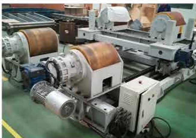
20t升降平移式滚轮架 20t conventional rotator(Horizontal moving and elevating)
