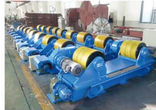
批量生产的200t丝杆可调式滚轮架（聚氨酯轮） 200t conventional power control turning-roll in batch production(polyurethane tire)
