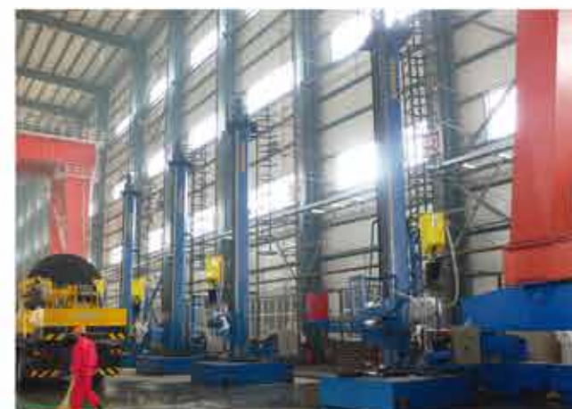
6m×5m重型焊接操作机（配林肯机头） 6m×5m heavy-duty welding manipulator(with LINCOLN head)
