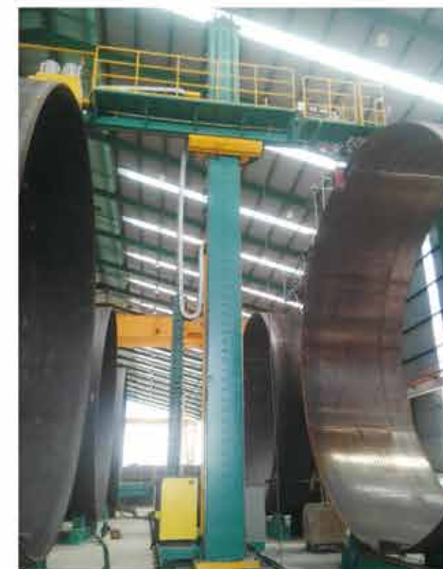
10m×7m超重型焊接操作机（带载人操作平台） 10m×7m super-heavy type welding manipulator(with manned platform)
