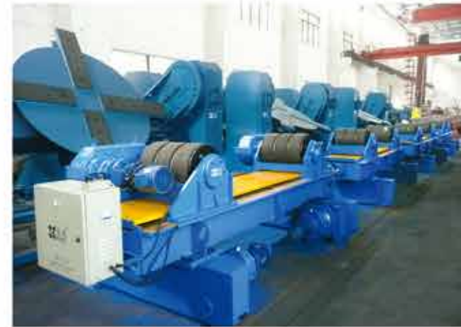
100t丝杆可调式滚轮架（带电动行走） 100t conventional power control turning-roll(Motorized travelling)
