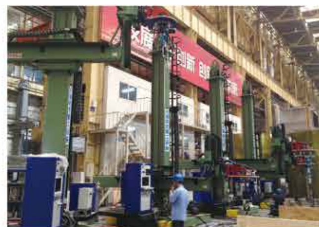
5*5 超重型操作机 (配宝利苏迪热丝TIG焊) 5*5 welding manipulator (Equipped with POLYSOUDE hot wire TIG welding)
