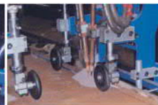
Twin wires with twin arc ( DC+AC )
