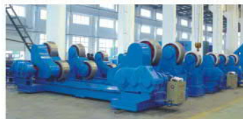
500 T SELF-ALIGNED WELDING ROTATOR
