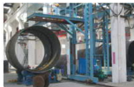
■ Circumferential seam welding
