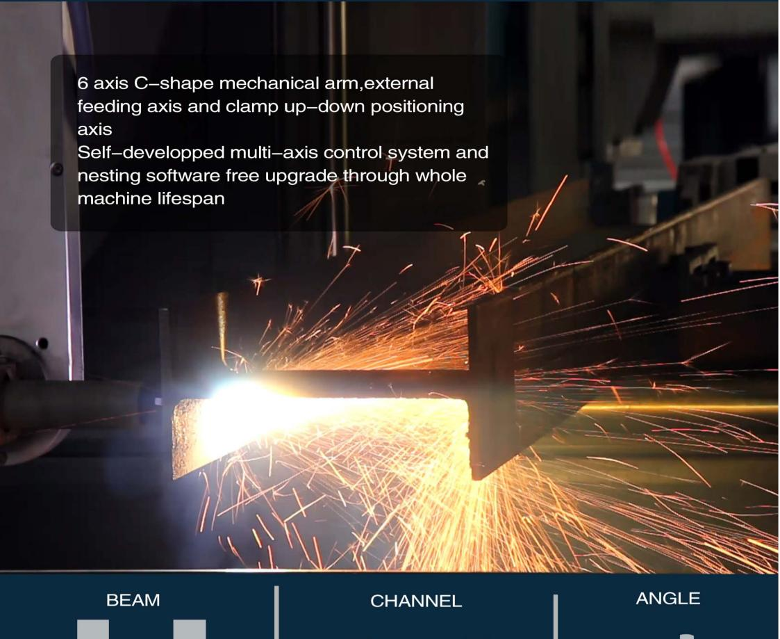
KR-XH600 KR-XH1000 KR-XH1500 Machine Min capacity Min capacity Min capacity Max capacity Max capacity Max capacity Mm(in) Mm(in) Mm(in) Mm(in) specifications Mm(in) Mm(in) width/height width/height width/height width/height Width/height width/height 100 (4) 100 (4) 1500(59) 600 (24) 1000(40) 100 (4) Beam 100 (4) Channel 600 (24) 100 (4) 700 (27) 100 (4) 1000(39) 100 (4) 1000(39) 100 (4) Angle 400 (16) 700 (27) 100 (4) **8T** 10T Load 12T
